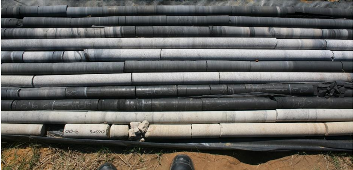
Figure 1: Example of a coal borehole core logged by a human expert based on what the human eye can observe (mainly brightness).
